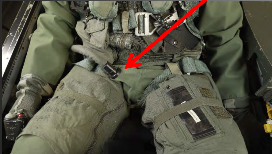
TSC is a one way check valve
