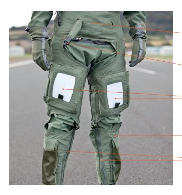
Bladder facilitates air passage to assist inflation. Extends across the abdomen and down each leg to ensure high manoeuvrability with up to 7g+ protection
